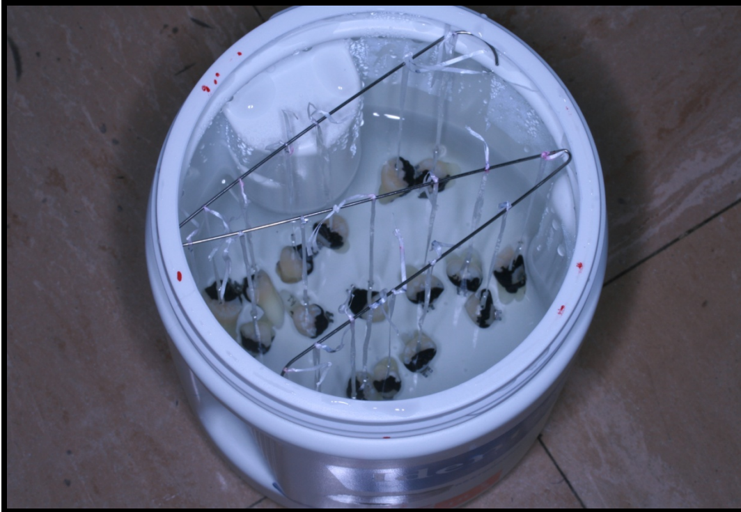
Figure 2: Group of teeth in the demineralization / remineralization solution.
